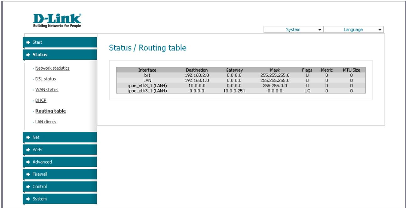
The screenshot shows the D-Link web interface for the DSL-2640U router. The page title is "Status / Routing table". On the left is a sidebar with a navigation menu. The main content area contains a table with the following data:
