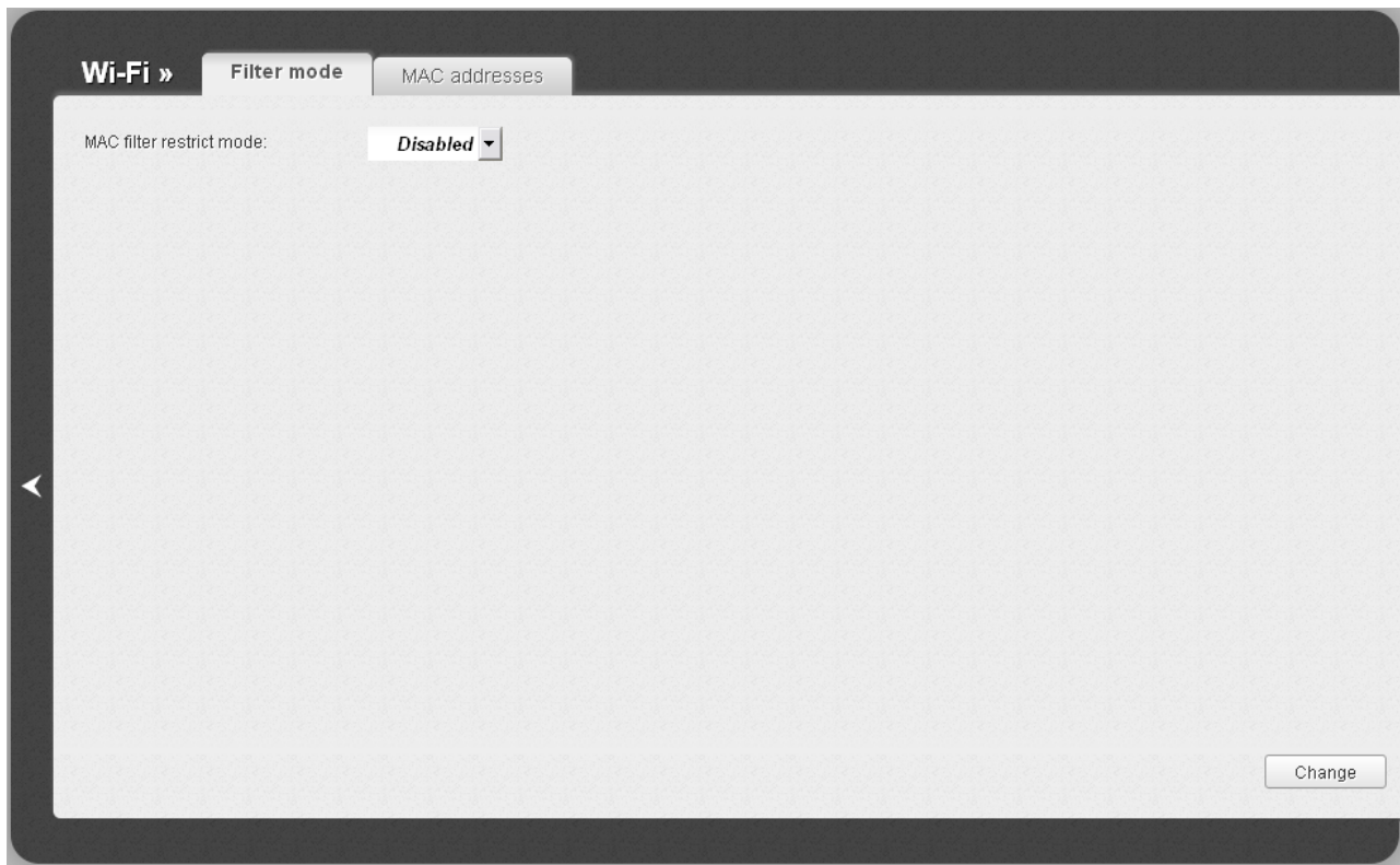
Figure 75. The MAC filter for the wireless network.
