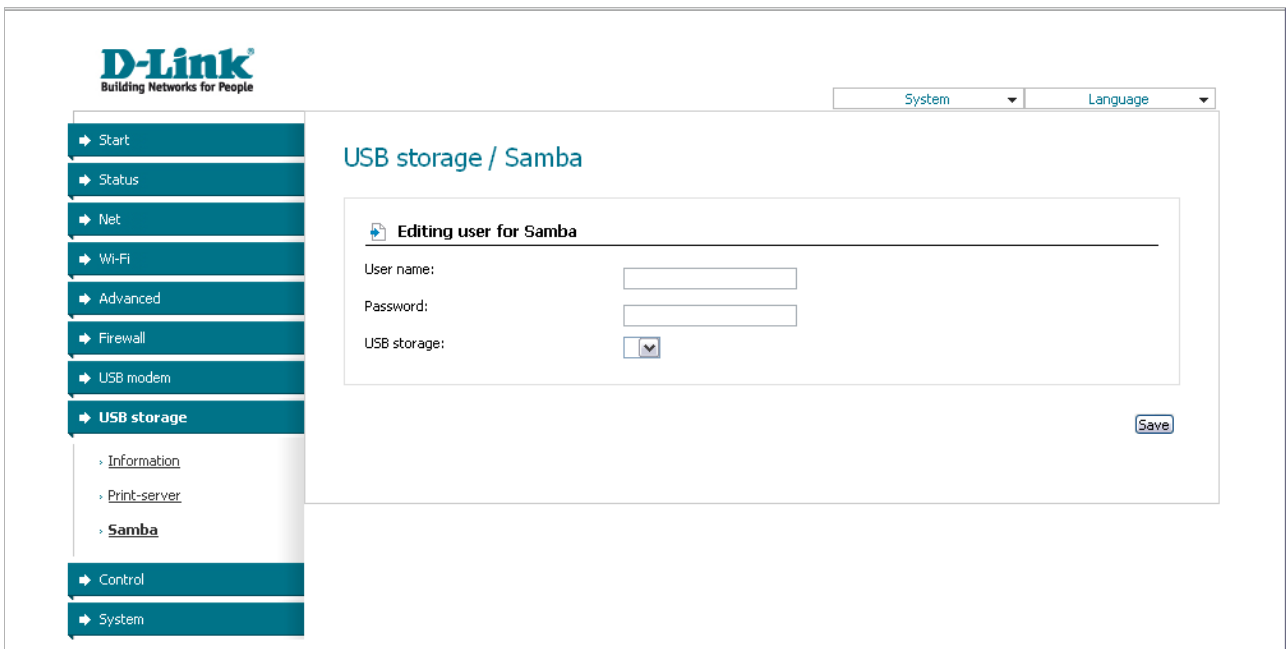
Figure 71. The page for adding an account used to access the USB storage.
