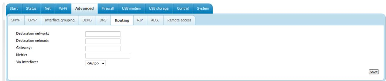
Figure 87. The page for adding a static route.
