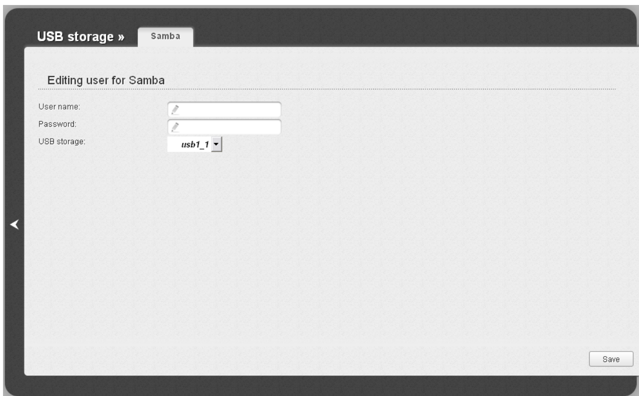
Figure 112. The page for adding an account used to access the USB storage.
