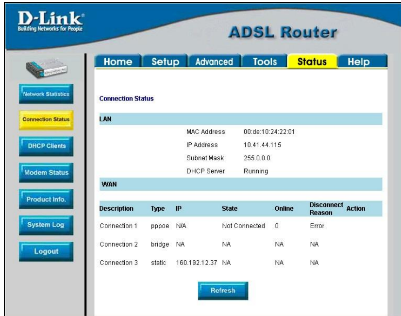
Figure 4-22. Connection Status window
