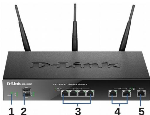
Figure 1. DSR-1000AC Front Panel
