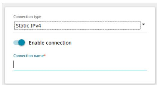
Figure 34. The page for creating a new **Static IPv4** connection. Selecting a connection type.
