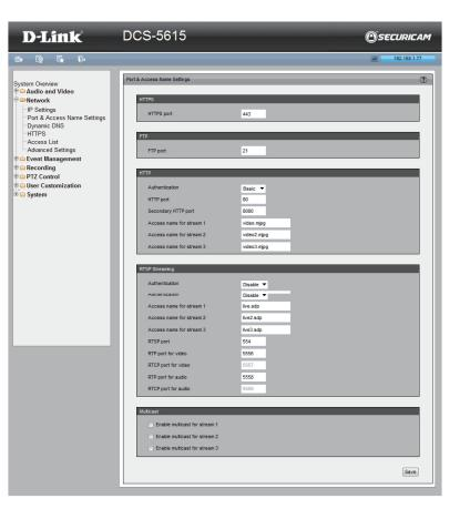
Access name for stream 1 ~ 3: This Network Camera supports multiple streams simultaneously. The access name is used to differentiate the streaming source. If you want to use an RTSP player to access the Network Camera, you have to set the video mode to H.264 / MPEG-4 and use the following RTSP URL command to request transmission of the streaming data. RTSP port /
