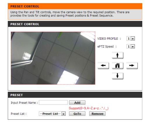
**Preset Sequence:** This section allows you to create a preset sequence, which automatically moves the camera's view between a set of preset views.
