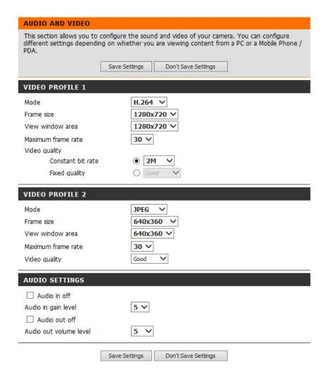
Video Quality: This limits the maximum frame rate, which can be combined with the "Fixed quality" option to optimize the bandwidth utilization and video quality. If fixed bandwidth utilization is desired regardless of the video quality, choose "Constant bit rate" and select the desired bandwidth.
