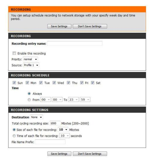
Total cycling Please input a HDD volume between 1MB and 2TB recording size: for recording space. The recording data will replace the oldest record when the total recording size exceeds this value. For example, if each recording file is 6MB, and the total cyclical recording size is 600MB, then the camera will record 100 files in the specified location (folder) and will then delete the oldest file and create new file for cyclical recording.
