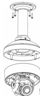
Place the camera body onto the bracket cap and attach the dome to the base of the camera using the four long screws and the security screw.
