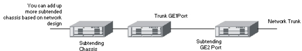
Figure 6-2 Daisy-Chain Topology for DAS-4192-10 NC Card
