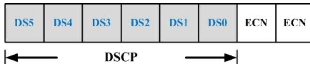
The most significant six bits of DiffServ field are called DSCP. The network device classifies packets and marks them with appropriate DSCP value. According to these values, other network devices in the DiffServ domain can make decision for packets behavior and provide the Quality of Service properly.
