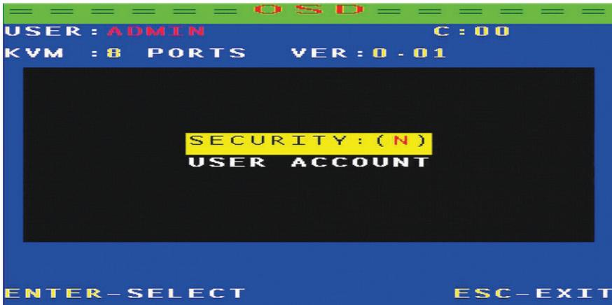
When you press F7 into the user settings, the screen shown in Figure 4, SECURITY: Y represents that need the password to enter, N on behalf of don't need the password to enter, press the "↓" into the user account, Press "enter" to into, enter the screen as Figure 5
