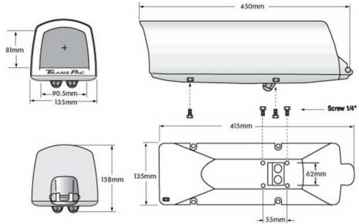
Camera mounting space (lens Incl.): 260 mm x 60mm x 80mm (L x W x H)
