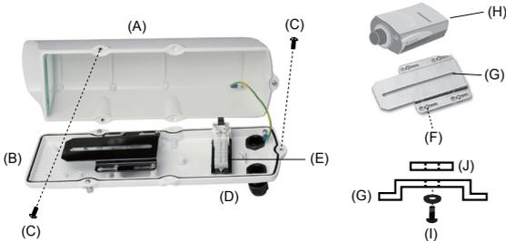
1. Unscrew the 3 captive **retaining screws** (C) and remove the **housing cover** (A) from the **housing base** (B).
