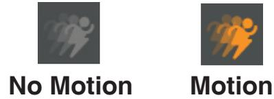
The motion notification will continue to blink as long as motion is detected. If no additional motion is detected, it will return to its original state after eight seconds.
