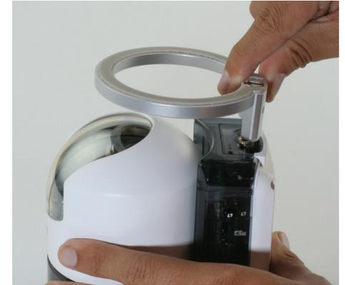
Tighten the nut on the top of the mounting stand using a coin or a screwdriver.
