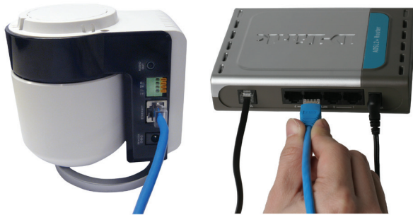
Connecting to a router
