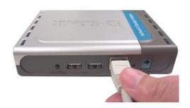
Attach the other end of the provided Ethernet cable to an available Ethernet port on your router or switch.
