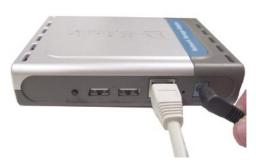
Attach your USB drive(s) to the USB port(s) on the rear panel of the DNS-120.
