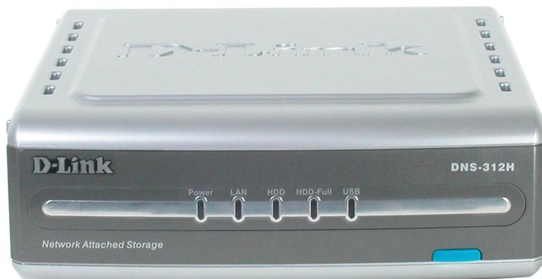
**Power:** A solid light indicates a proper connection. No light indicates the power is off.
