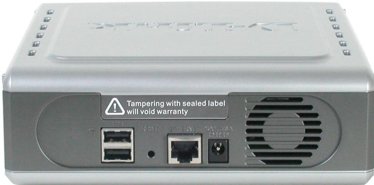
**USB Ports for Printer Server/USB HDD:** Please use the USB printer cable to connect the DSM-312H's USB Port (for printer server) or USB HDD for additional volume.
