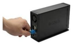
Note: Should you need to install a new Hard Disk into the DNS-313, you will be required to insert the Ethernet cable between your DNS-313 and router and run the original DCC installation wizard included in the CD **Please do not connect the USB cable during this step.**
