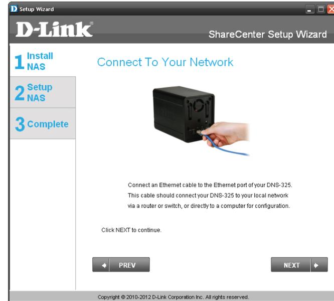
**Step 6** - Connect a CAT5 Ethernet cable with RJ-45 connectors to your ShareCenter™ and connect the other end to a switch or router (Local LAN).
