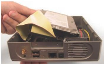
Use the mounting screw to secure the hard drive to the DSM-600. Replace the cover and screw the two screws on the back panel of the DSM-600.
