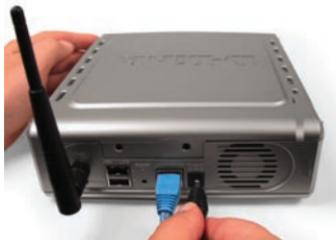
**Note:** When you first power on and access the Web-Interface, the DSM-600 will offer to format your hard drive if it is unformatted. This process may take several minutes depending on the size of your hard drive. During this process, the power LED will blink. Do not power the unit off during the formatting process. Once the power LED is solid, you may then access the web based configuration of the DSM-600.
