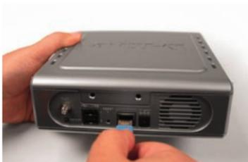
**Note:** It is required that an Ethernet cable is used during initial setup.
