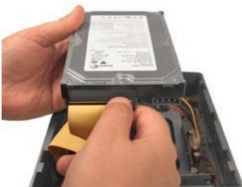
Connect the power cable to the power connector on your hard drive.
