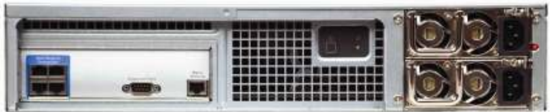
Figure F- 2 Rear View of Enclosure
