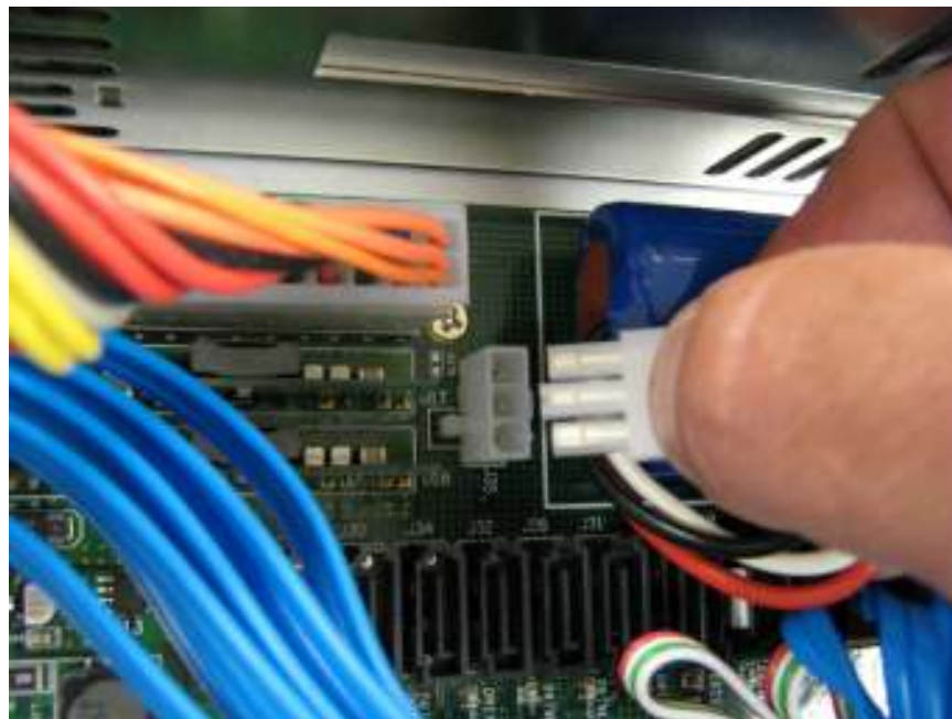
Figure D-3 Align the Battery Plug with Connector J35
