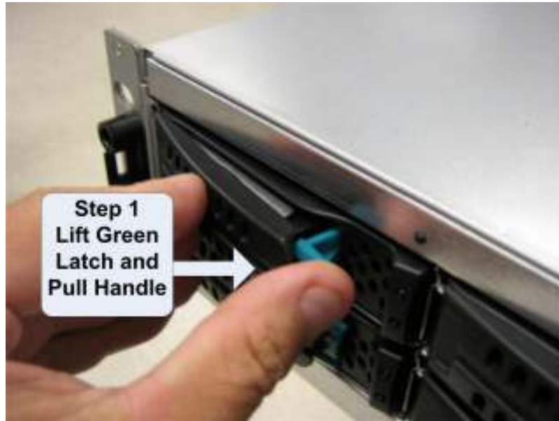
Figure 2-2 Drive and Tray Removal
