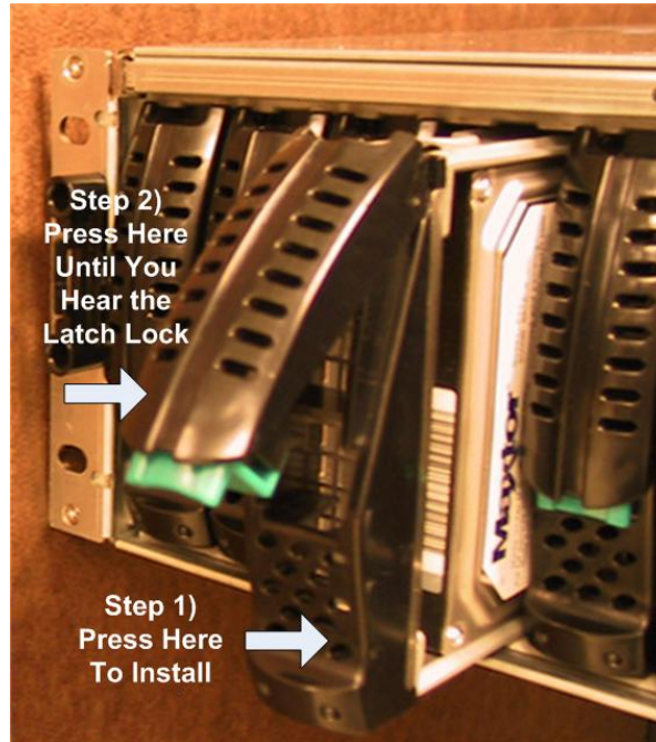
Figure 3-3 Drive and Tray Installation
