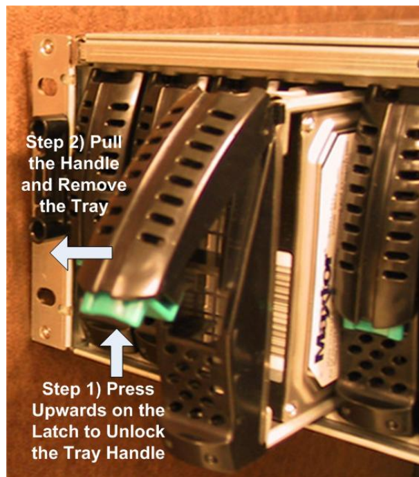
Figure 3-2 Drive and Tray Removal
