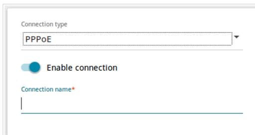
Figure 70. The page for creating a new **PPPoE** connection. Selecting a connection type.
