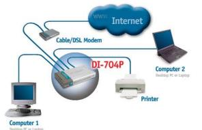
With the DI-704P you can share Internet access and resources such as printers in your home or office. Connect up to four computers and a printer with the DI-704P's parallel printer port.
