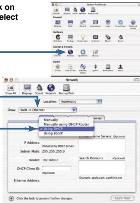
The IP address information, the Subnet Mask, the Router's IP address and the Ethernet adapter address will appear.
