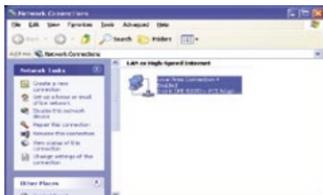
For **Microsoft Windows XP**: Go to **Start > right click on My Network Places > select Properties > Right click on the Network Connection associated with the Ethernet adapter and select Properties** (i.e., D-Link DFE-530TX+).
