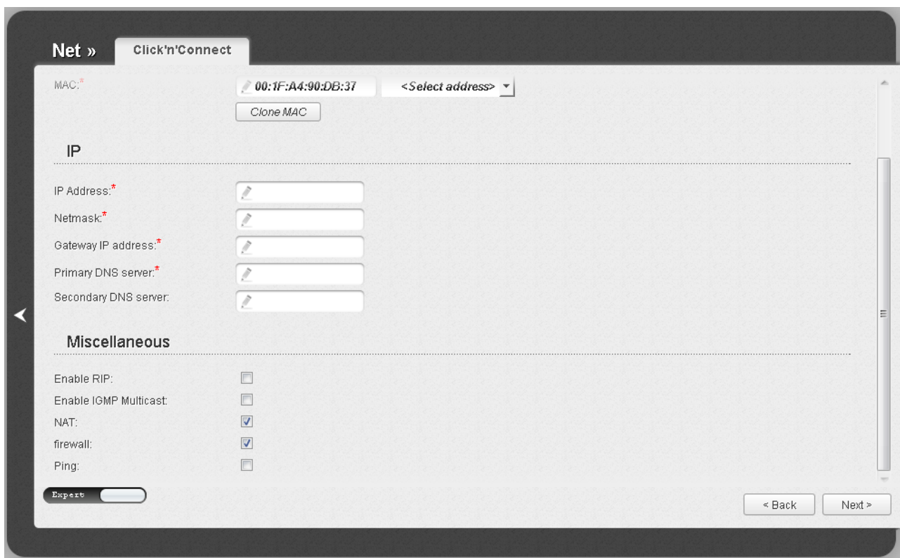
Figure 38. Configuring PPTP + Static IP WAN connection. The expert settings mode. The IP and Miscellaneous sections.
