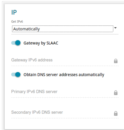
Figure 74. The page for creating a new PPPoE IPv6 connection. The IP section.
