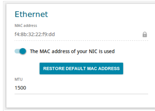
Figure 72. The page for creating a new PPPoE IPv6 connection. The Ethernet section.
