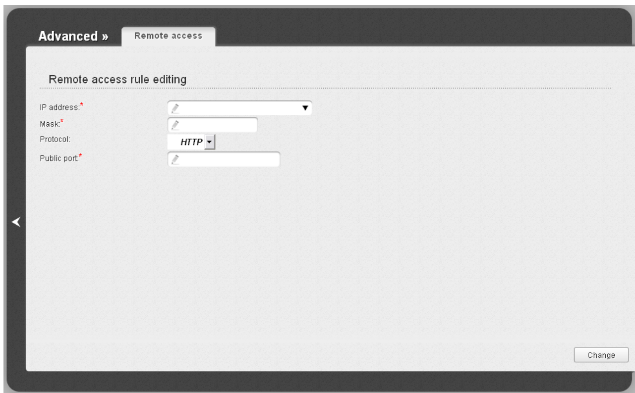
Figure 113. The page for adding a rule for remote management.
