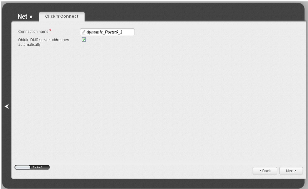
Figure 33. Configuring Dynamic IP WAN connection.
