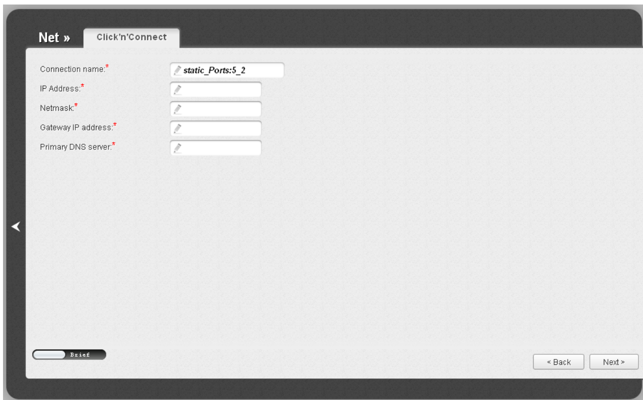
Figure 30. Configuring Static IP WAN connection.
