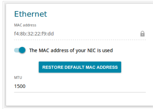
Figure 58. The page for creating a new Static IPv4 connection. The Ethernet section.
