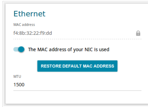
Figure 73. The page for creating a new PPPoE IPv6 connection. The Ethernet section.
