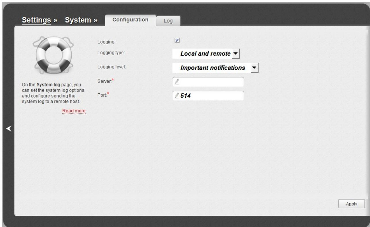
Figure 120. The **System / System log** page. The **Configuration** tab.
