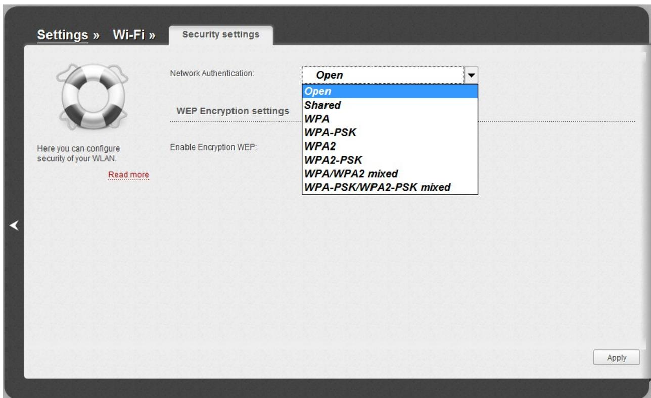
Figure 89. Network authentication types supported by the router.
