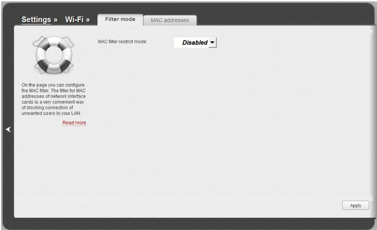
Figure 93. The MAC filter for the wireless network.
