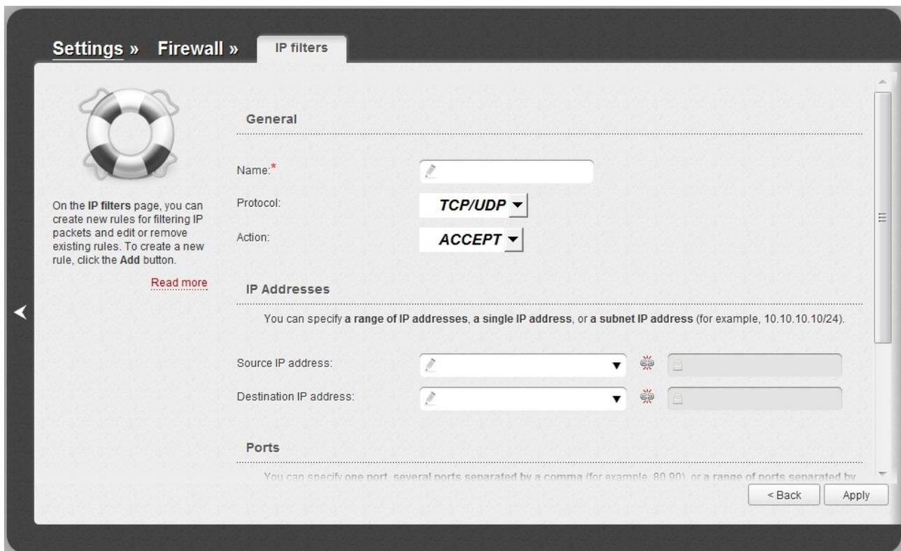
Figure 111. The page for adding a rule for IP filtering.
