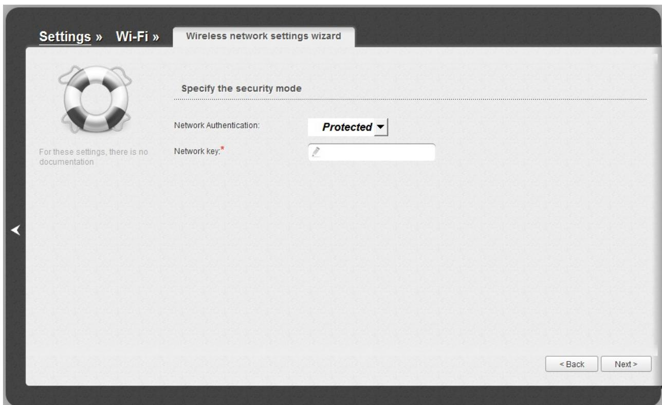
Figure 58. Page for selecting a security mode for the wireless network.
