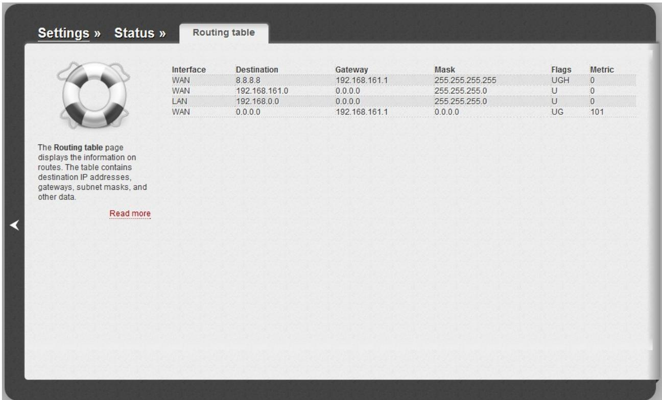
The screenshot shows the 'Routing table' page in the router's web interface. At the top, there is a breadcrumb trail: 'Settings » Status » Routing table'. Below this, there is a lifebuoy icon. To the right of the icon is a table with the following data:
