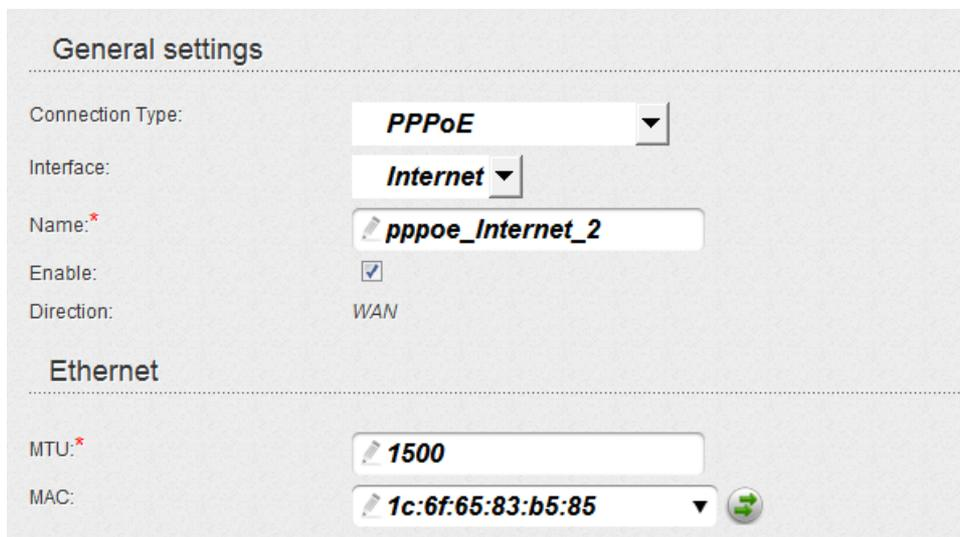
The screenshot shows a configuration page with two main sections: **General settings** and **Ethernet**. In the **General settings** section, the **Connection Type** is set to **PPPoE**, the **Interface** is **Internet**, the **Name** is **pppoe\_Internet\_2**, the **Enable** checkbox is checked, and the **Direction** is **WAN**. In the **Ethernet** section, the **MTU** is set to **1500** and the **MAC** address is **1c:6f:65:83:b5:85**.
