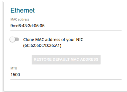
Figure 69. The page for creating a new PPPoE IPv6 connection. The Ethernet section.
