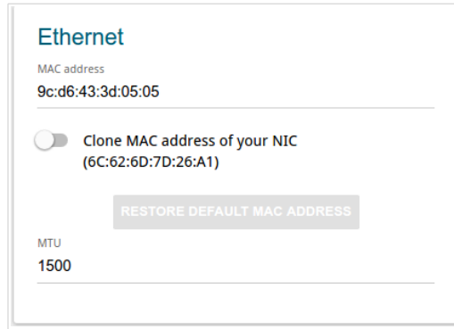
Figure 54. The page for creating a new Static IPv4 connection. The Ethernet section.
