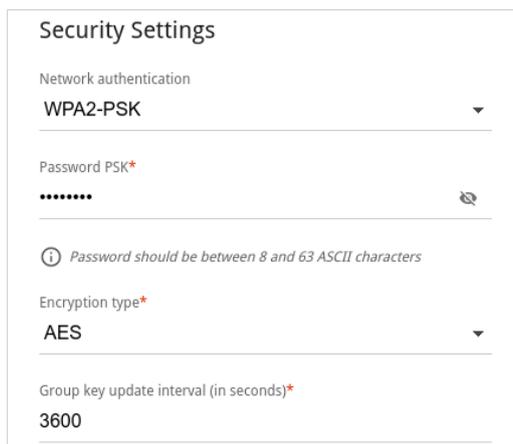
Figure 80. The **WPA2-PSK** value is selected from the **Network authentication** drop-down list.
