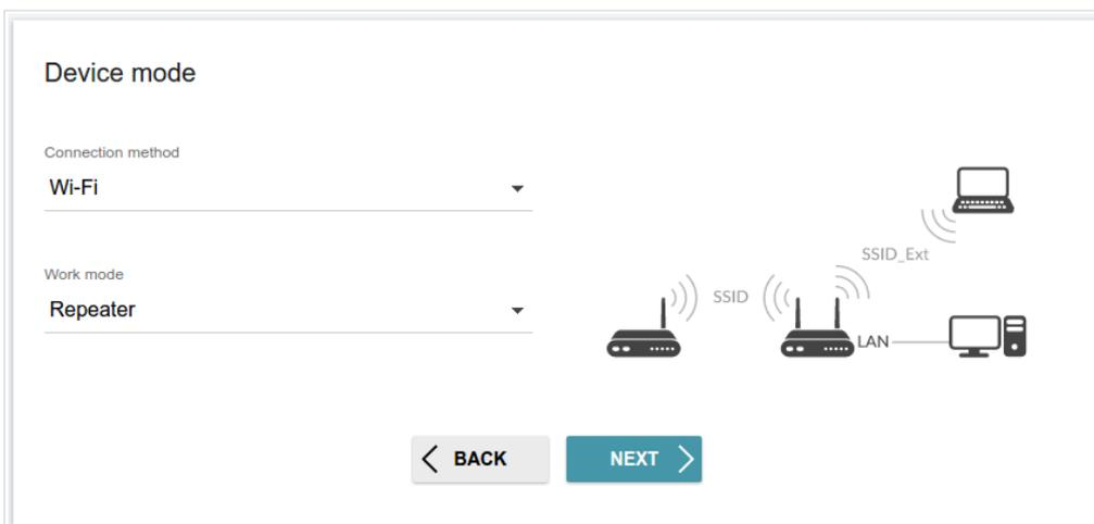
Figure 38. Selecting an operation mode. The **Repeater** mode.
