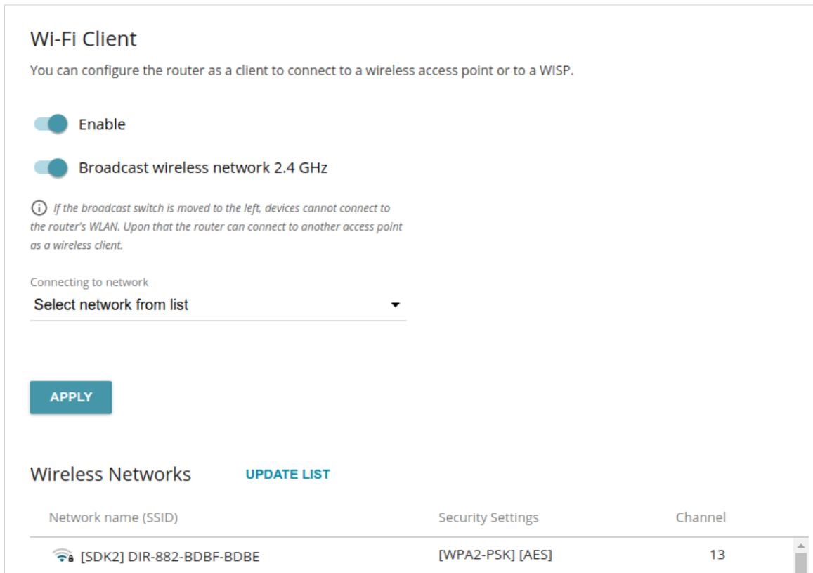
Figure 101. The page for configuring the client mode.
