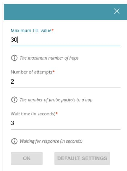
Figure 141. The **Management / Diagnostics / Traceroute** page. The additional settings window.
