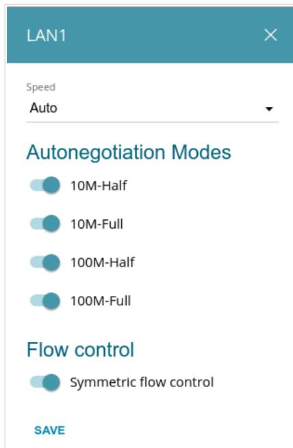
Figure 120. The window for changing the settings of the router's port.
