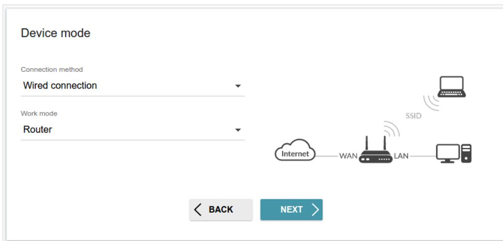
Figure 35. Selecting an operation mode. The **Router** mode.
