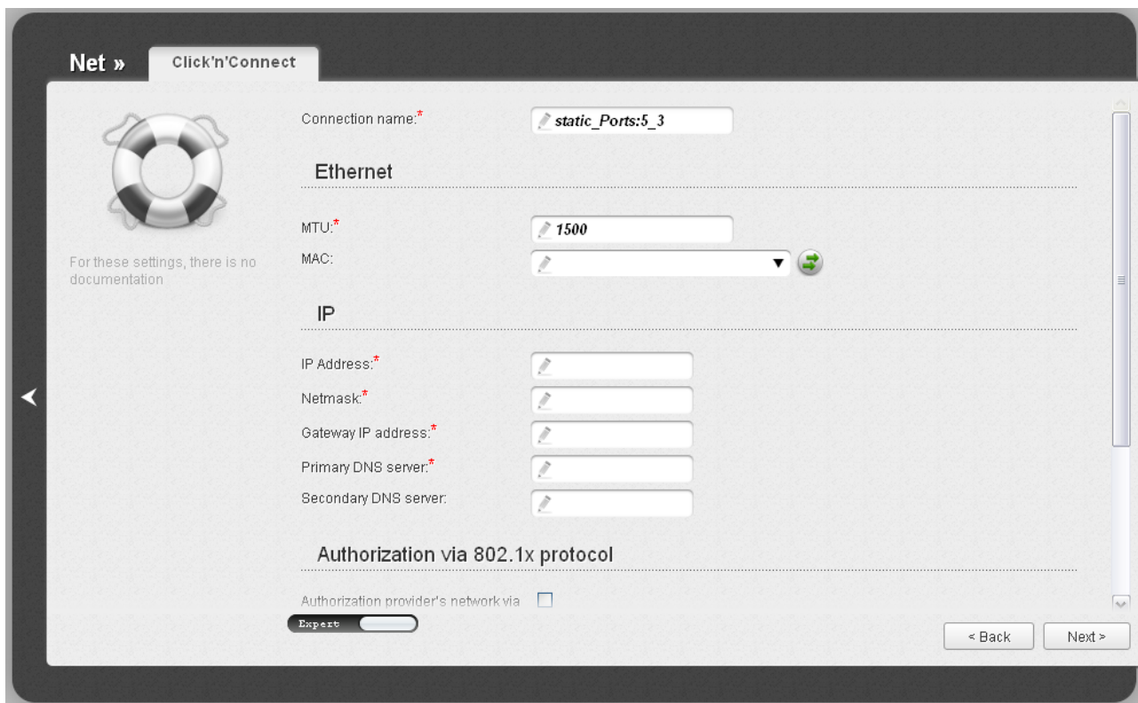
Figure 32. Configuring Static IP WAN connection. The expert settings mode. The Ethernet section.
