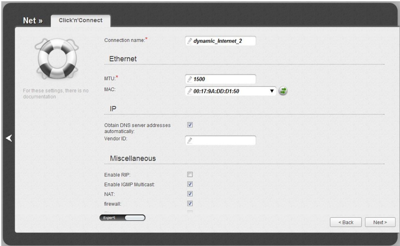
Figure 35. Configuring Dynamic IP WAN connection. The expert settings mode. The Ethernet section.
