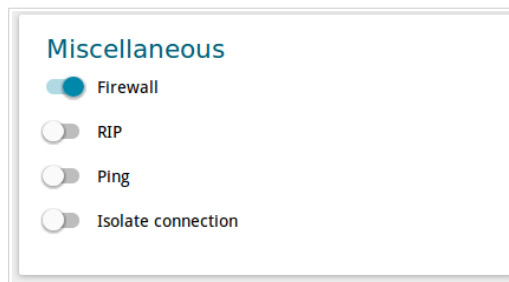
Figure 78. The page for creating a new PPPoE IPv6 connection. The Miscellaneous section.
