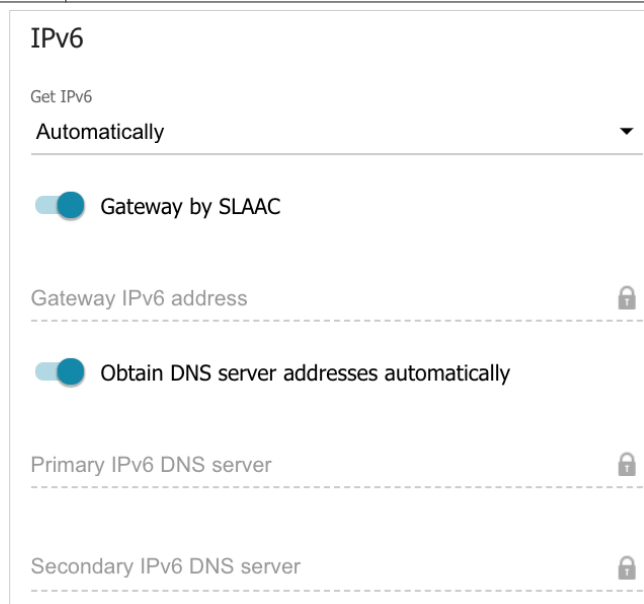
Figure 78. The page for creating a new PPPoE Pv6 connection. The IPv6 section.
