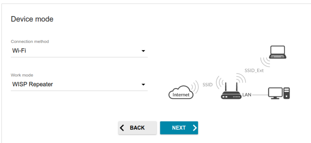
Figure 34. Selecting an operation mode. The WISP Repeater mode.
