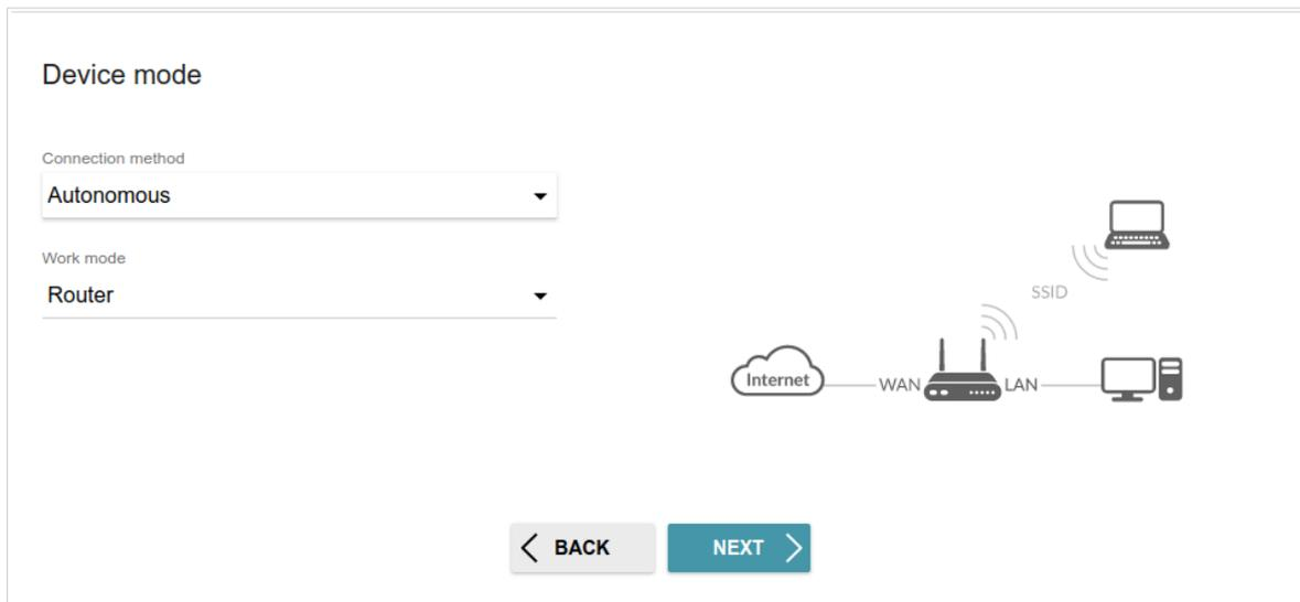
Figure 36. Selecting an operation mode. The **Router** mode.
