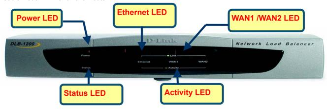
The corresponding Ethernet Indicator should be ON while a PC connected to the Ethernet Port. If any error condition shows up, the Error Indicator stays ON.
