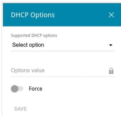
Figure 93. Configuring the local interface. The **IPv4** tab. The window for configuring a DHCP option.
