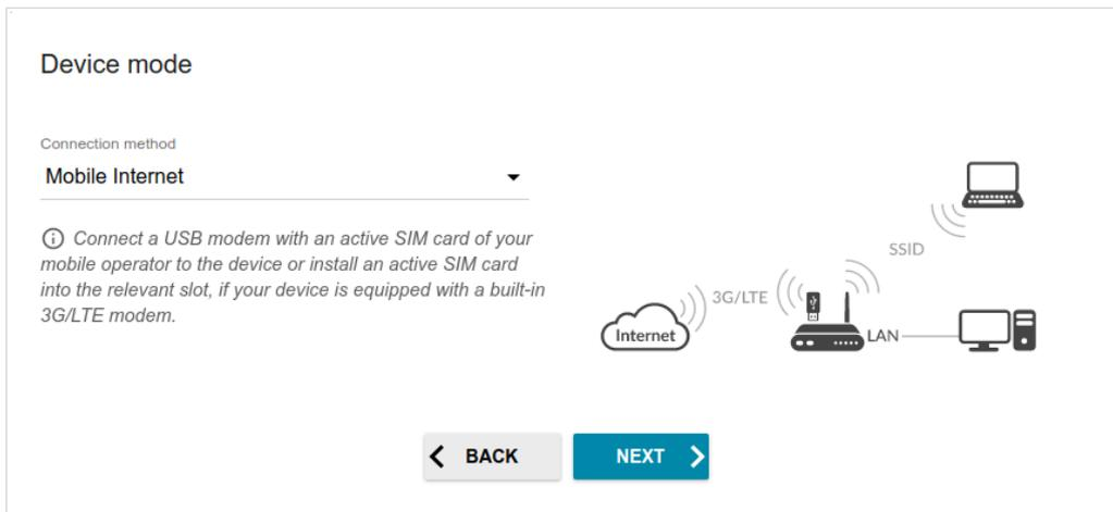
Figure 34. Selecting an operation mode. The **Mobile Internet** method.
