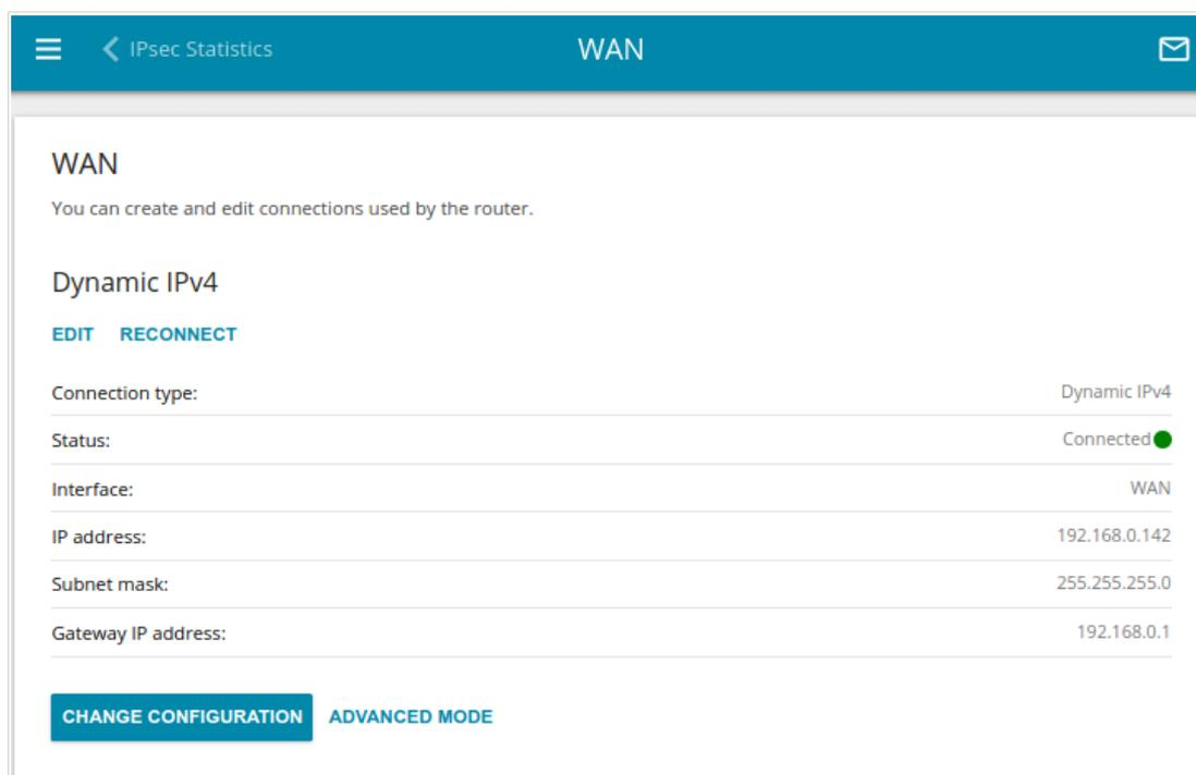
Figure 58. The **Connections Setup / WAN** page. The simplified mode.
