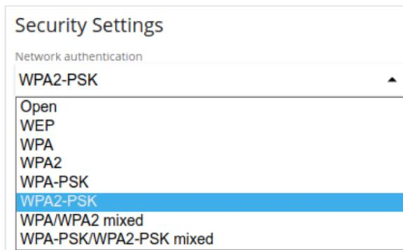
Figure 123. Network authentication types supported by the router.
