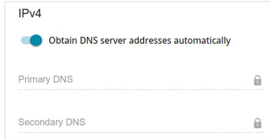
Figure 78. The page for creating a new **PPPoE Dual Stack** connection. The **IPv4** section.
