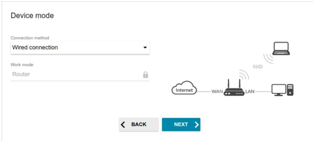
Figure 33. Selecting an operation mode. The **Wired connection** method.
