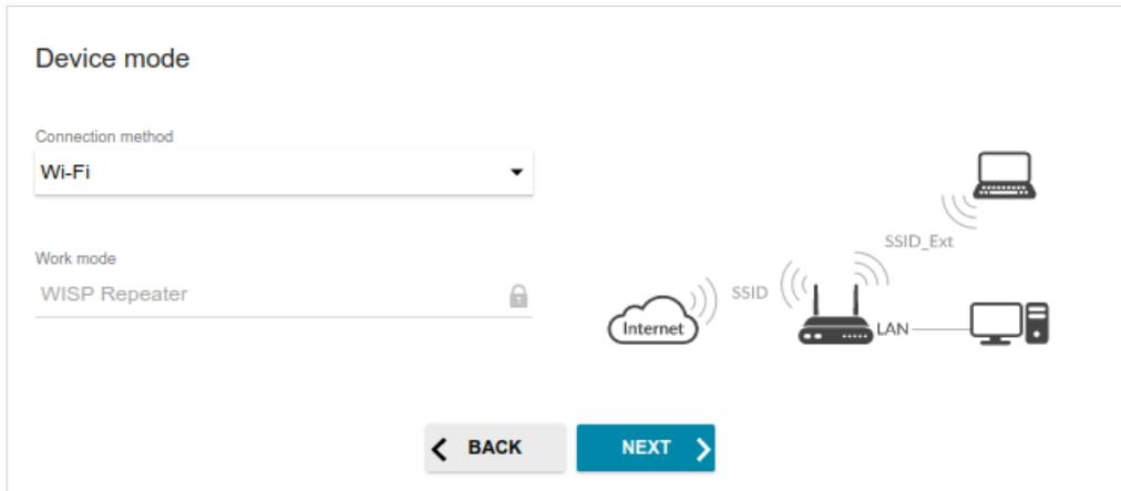
Figure 35. Selecting an operation mode. The **Wi-Fi** method.
