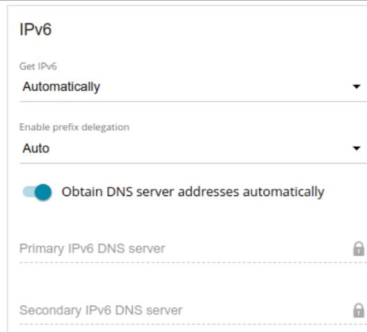
Figure 79. The page for creating a new **PPPoE Pv6** connection. The **IPv6** section.
