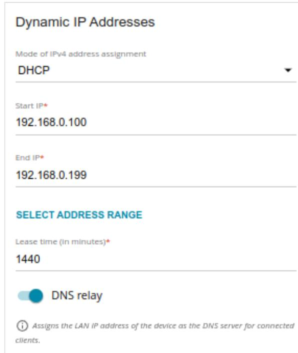
Figure 91. Configuring the local interface. The IPv4 tab. The **Dynamic IP Addresses** section.
