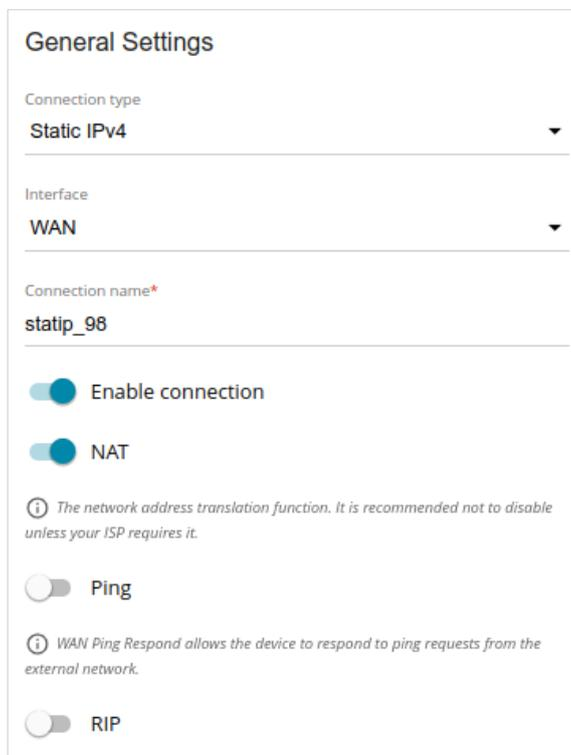
Figure 60. The page for creating a new **Static IPv4** connection. The **General Settings** section.
