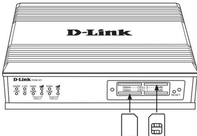
Figure 5: Installing a SIM card
