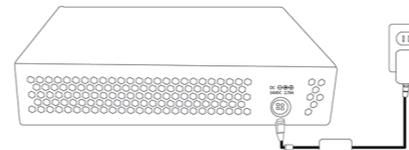
Figure 2. Plugging the switch into an outlet
