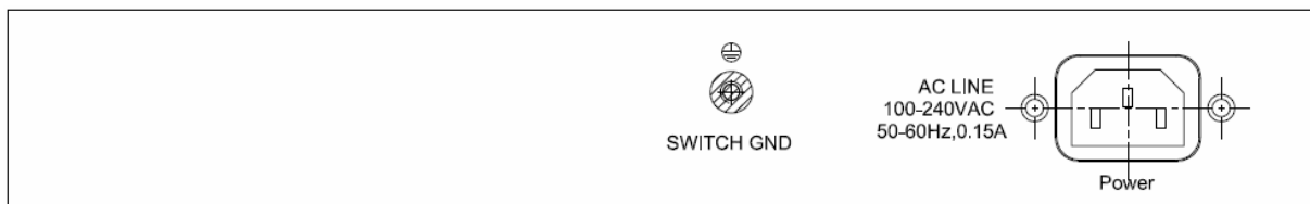
Figure 2 – DES-1100-16 Rear Panel
