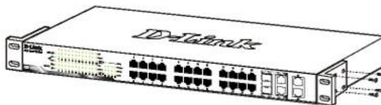
Figure 10 – Attach the mounting brackets to the Switch
