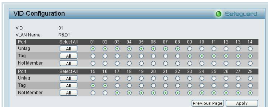
Figure 65 – Configuration > 802.1Q VLAN > VID Assignments
