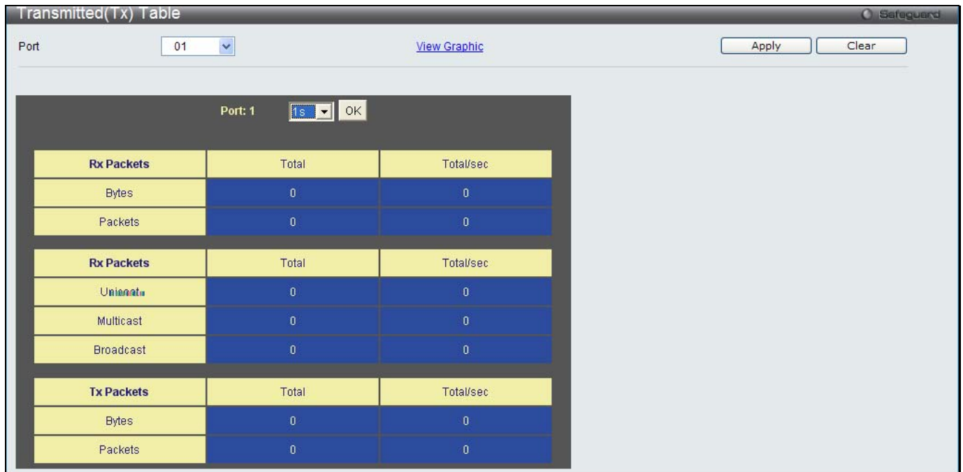
Figure 7 - 12. Transmitted (Tx) Table window (for Bytes and Packets)
