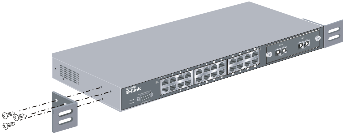
Figure 2-5. Attach mounting brackets
