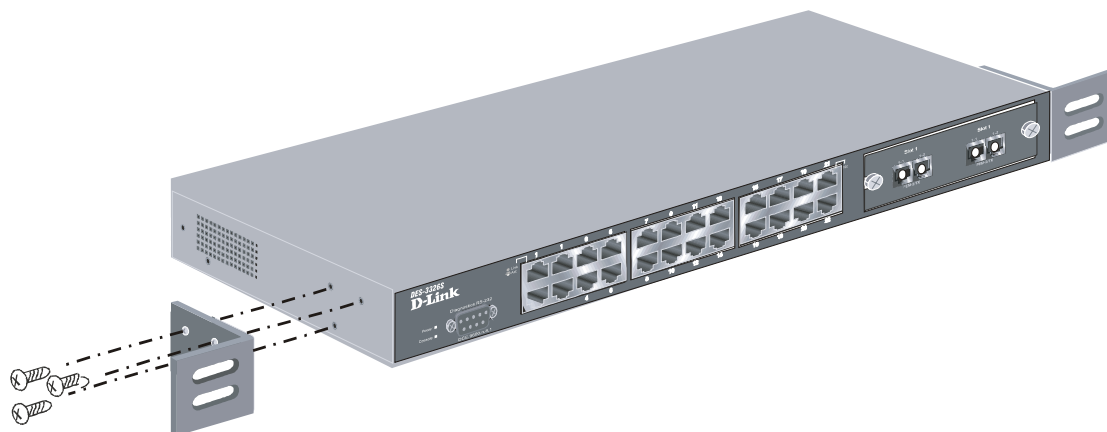
Figure 2-5. Attach mounting brackets
