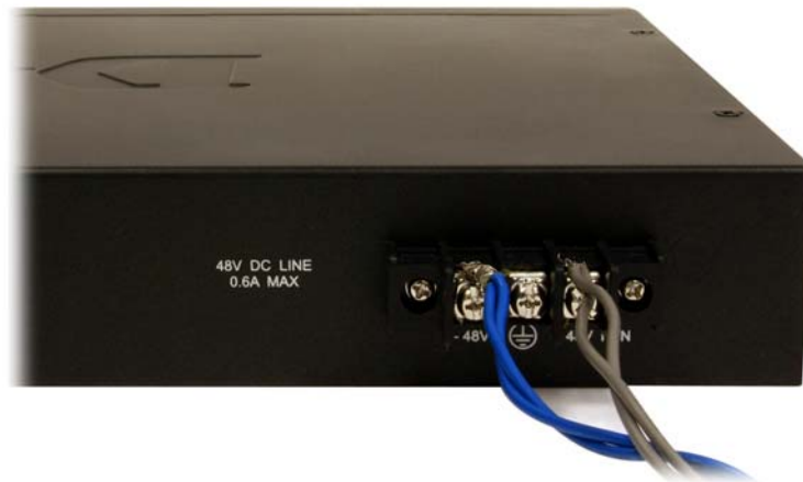
Figure 2- 4. Power connections attached to contacts after assembly
